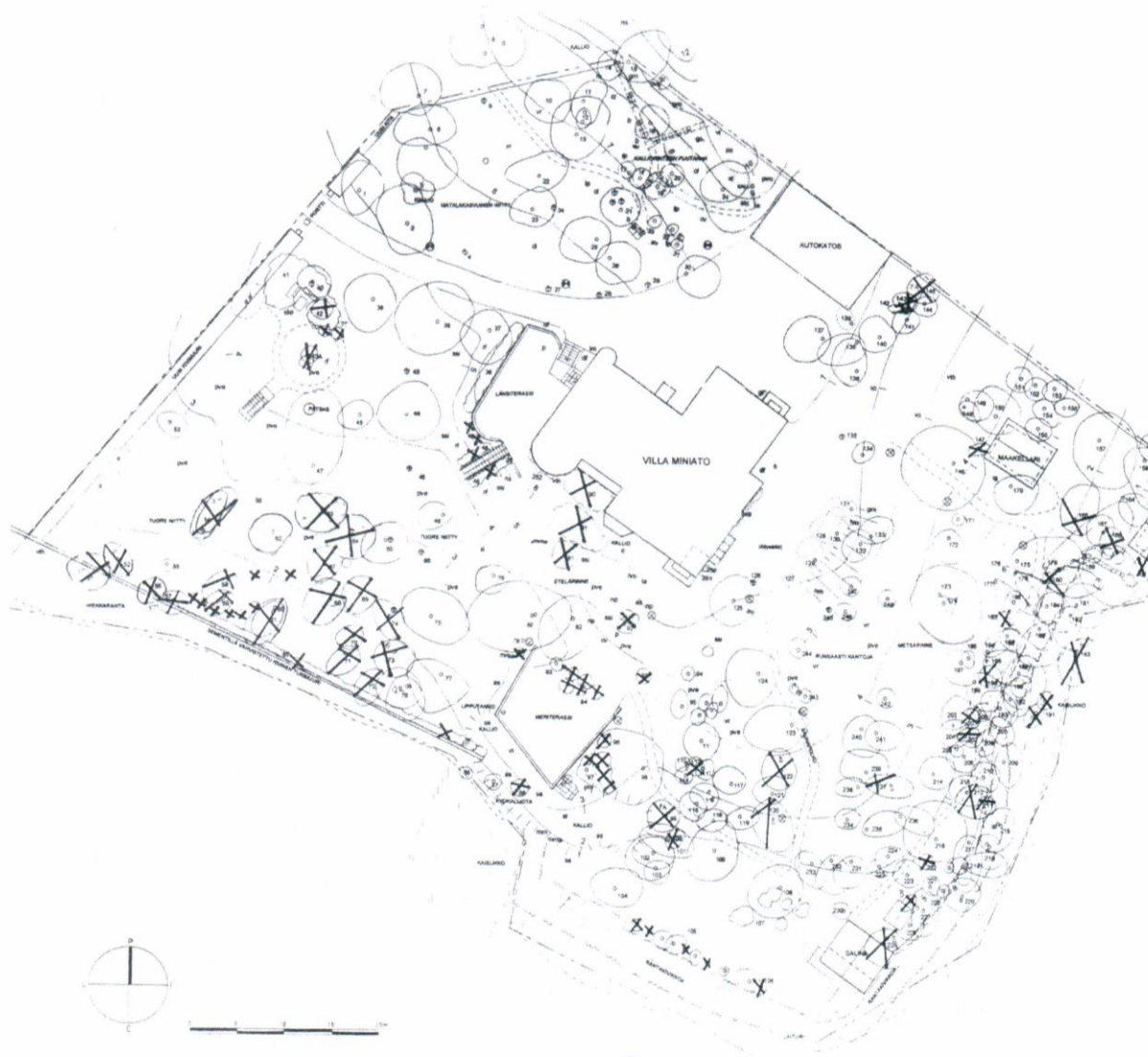
Appendix 6 A tree-felling plan on 3/23/2001, drawing No. 122-02, a small-scale map also including a plant-specific table, Molino Oy, Minna Piispanen.
